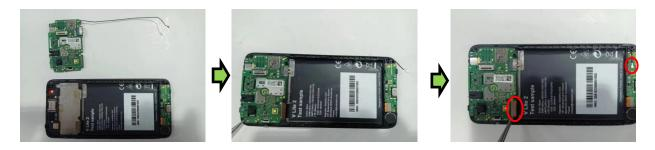
Assemble the PCBA by using the forceps and install the LCD FPC &SIDEKEY FPC&RF Cable connection.
