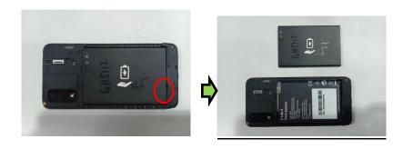
Remove the the battery carefully.
