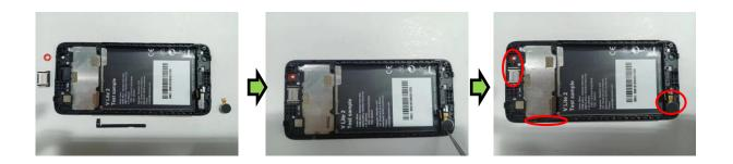
Assemble the Speaker & SIDEKEY FPC & Motor&Front camer rubber in the upper housing.
