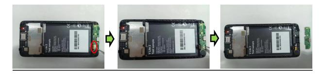
Use the forceps open the SUB FPC connection, remove the SUB PCB from the upper housing assembly.
