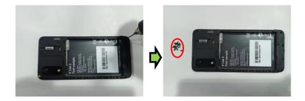
Remove the screws (qty=13) by using the screwdriver carefully.
