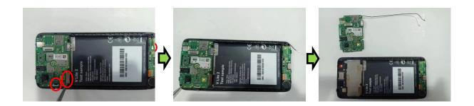
Use the forceps to open the LCD FPC &SIDEKEY FPC&RF Cable connection and remove the PCBA from the upper housing.
