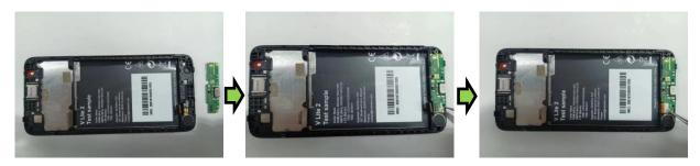
Assemble the REF SUB by using the forceps and install the SUB FPC connection.
