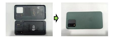
Assemble the battery cover carefully .
