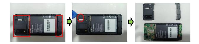
Insert a rigid thing plastic card between the lower1 and upper housing assembly. Start from the bottom of the product, then continue on the sides and remove carefully the lower1 housing assembly.Remove the lower2 in the same way.
