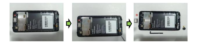
Remove the Speaker & SIDEKEY FPC & Motor&Front camer rubber from the upper housing.
