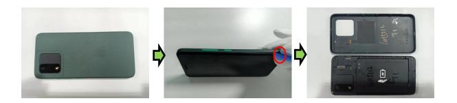
Remove the battery cover by opening the special slot.
