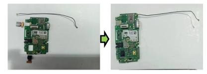
Assemble the Front camera&Back camera &RF Cable by using the forceps and keep carefully.
