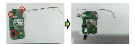
Remove the Front camera & Back camera & RF Cable from the PCBA.
