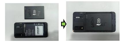
Assemble the battery carefully.
