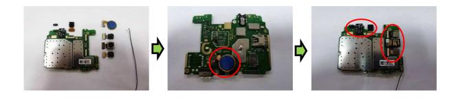
Assemble the Back camera(qty=3) and Front camera.RF Cable.Sensor rubber.Fig by using the forceps and keep carefully.
