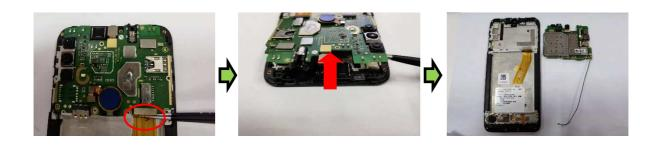
Use the forceps to open the LCD FPC connection and remove the PCBA from the upper housing.
