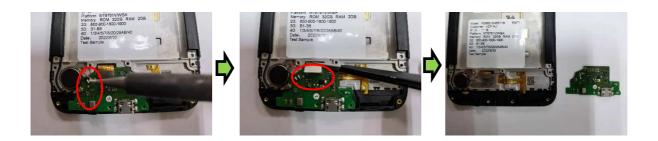
Use the forceps and soldering iron to open the SUB FPC connection and motor connection and remove the SUB PCB from the upper housing assembly.
