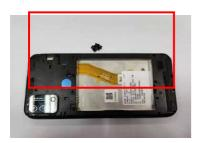
Remove the screws (qty=18) by using the screwdriver carefully.
