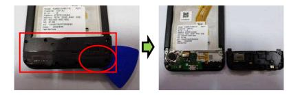
Insert a rigid thing plastic card between the lowerB and upper housing assembly. Start from the bottom of the product, then continue on the sides and remove carefully the lowerB housing assembly.
