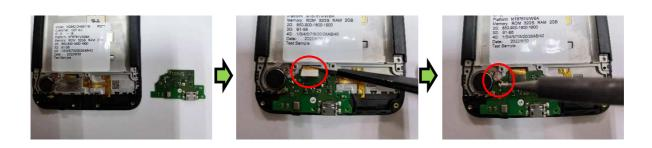
Assemble the REF SUB by using the forceps and install the FPC connection and RF Cable connection.
