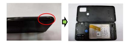
Remove the battery cover by opening the special slot.
