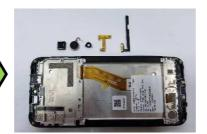
Remove the Receiver. FPC sidekey and Camera rubber. Spk fpc. Motor from the upper housing.
