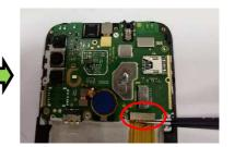
Assemble the PCBA by using the forceps and install the LCD FPC connection.
