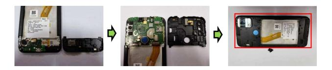
Assemble the Lower Housing A & Lower Housing B and fix it with the referenced screws (Qty =18).
