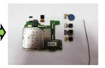
Remove the Back camera(qty=3) and Front camera.RF Cable.Sensor rubber.Fig from the PCBA.
