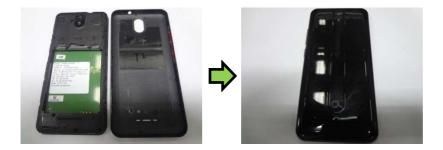
Assemble the battery cover carefully .
