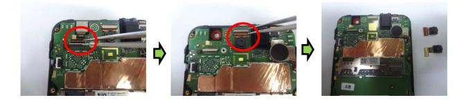
Remove the back camera and front camera by opening the connector.
