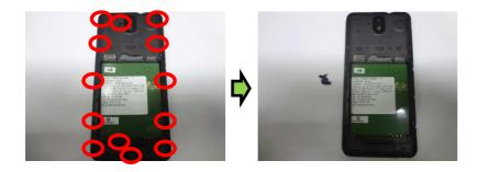
Remove the screws (qty=13) by using the screwdriver carefully.
