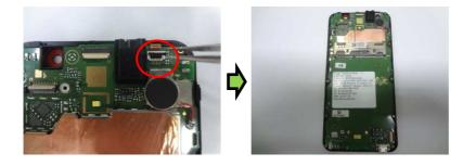
Use forceps and insert the LCD FPC. SIDEKEY FPC. TP FPC into the dedicated connector on the PCBA.
