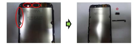
Remove the FPC SIDEKEY and receiver , Front camera rubber from the upper housing assembly by using the forceps.
