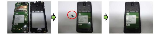
Assemble the Lower Housing and fix it with the referenced screws (Qty =13).
