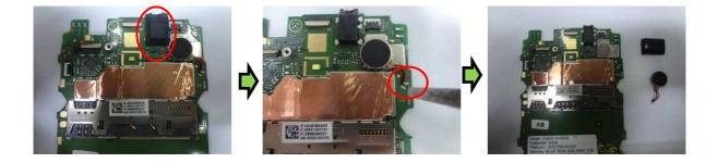
Take down the motor by using the soldering iron, and Earphone rubber.
