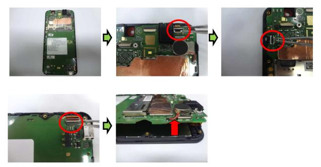
Open the LCD FPC connector and TP connector. FPC SIDEKEY connector by using the forceps.
