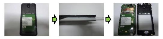
Insert a rigid thin plastic card between the lower and upper housing assembly. Start from the bottom of the product and along the sides to remove the lower housing assembly carefully.
