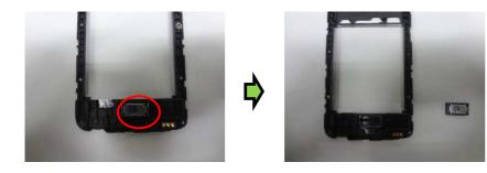
Remove the speaker from the lower housing assembly by using the forceps.
