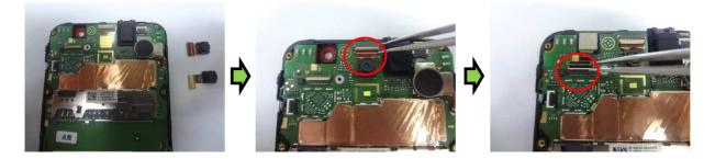
Assemble front camera and rear camera.
