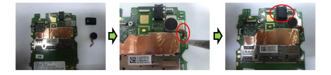
Assemble motors by using soldering iron and Earphone rubber.
