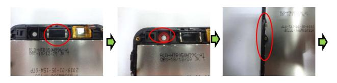
Use the forceps to put the receiver. FPC SIDEKEY. Front camera rubber in the special slot of the upper housing assembly.
