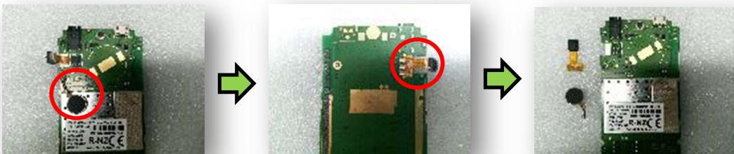
Remove the camer and Motor from the PCBA by using the soldering iron.
