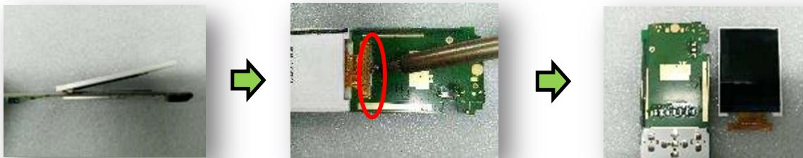
Remove the LCD from the PCBA by using the soldering iron.
